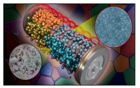
Oak Ridge National Laboratory (ORNL) scientists found that a small tweak created big performance improvements in a type of solid-state battery, a technology considered vital to broader electric vehicle adoption. These batteries use a solid electrolyte instead of a potentially flammable liquid. When the battery charges or operates, ions move between electrodes through the electrolyte between them.
