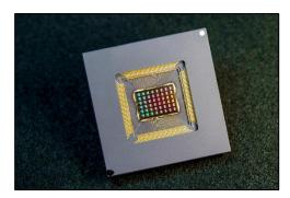
NeuRRAM, a new chip that runs computations directly in memory and can run a wide variety of AI applications has been designed and built by an international team of researchers. What sets it apart is that it does this all at a fraction of the energy consumed by computing platforms for general-purpose AI computing.
